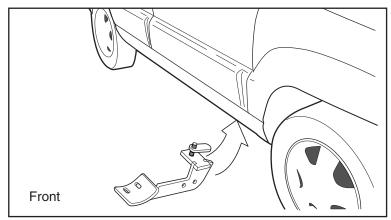
2. Lift pre-assembled bracket into position and insert threaded plate into opening.
