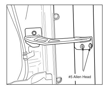
NOTE: Do not fully tighten hardware until the front is completed. Then follow the torque specifications listed below.
