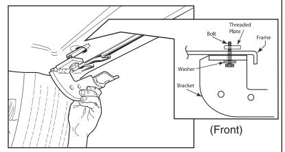
3. Remove two bolts from outer edge of heat shield and retain. Loosen two remaining bolts.
